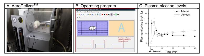
**A.** A rat inside the aerosol delivery chamber. **B**. The Operating program CageCenter. **C**. Data showing that the aerosol chamber delivers nicotine with results similar to the kinetic profile of human cigarette smoking.
